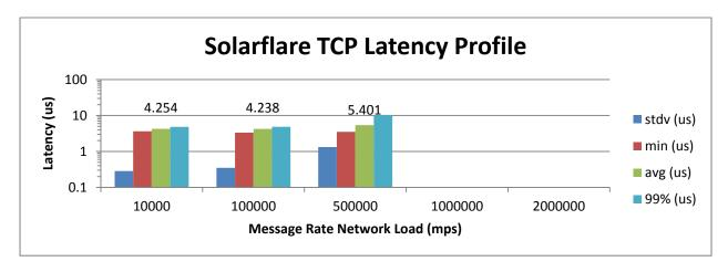
Again, the Solarflare adapter is not capable of sustaining high network loads without drops, therefore the missing datapoints at 1M and 2MPPS. The results are worse than for UDP, with higher latency and worse variance at any particular load point.
