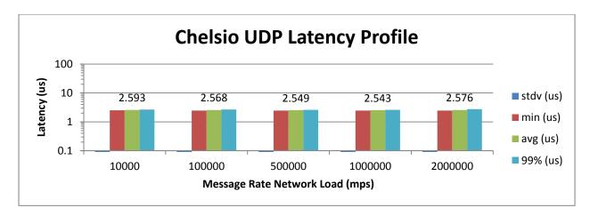
In contrast, Chelsio's solution is capable of sustaining loads in excess of 2MPPS, more than twice the limit of Solarflare. In addition, Chelsio's performance profile shows a remarkably consistent performance level, with minimum, average and 99% data points virtually indistinguishable, showing high tolerance for network load. This is a key difference between the two adapters, and can translate to dramatic difference in returns in actual HFT applications.
