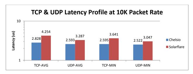
Chelsio's solution is as much as 1.4us lower latency than Solarflare at 10K packet rate. The latency under load test is a more realistic measure for latency in a typical HFT environment than a test with 1 packet in flight.
