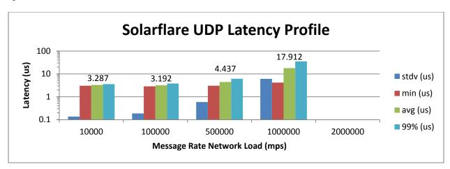
The Solarflare adapter is not capable of sustaining network loads at more than 1MPPS without dropping packets, therefore the missing datapoint at 2MPPS. Furthermore, its latency profile deteriorates significantly as the load is increased, along with increased variance, symptomatic of decreased stability as the capacity limit is approached.
