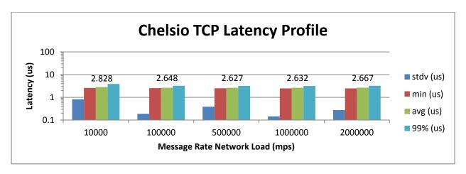
The figure above comparing WD-TCP and TCP Onload shows similar conclusions to the ones for UDP. Chelsio's solution offers a latency advantage that is maintained as the load is increased, and demonstrates much higher capacity at high load.
