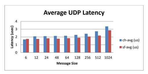
The test results show that Chelsio and Solarflare offer comparable UDP latency results in ping pong tests (single packet in flight). However, as shown in the previous section, when ingress rates are increased, Chelsio's performance is clearly superior, and extends to much higher loads.
