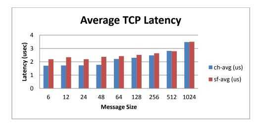
Chelsio provides better results than Solarflare in the TCP test. Furthermore, as shown in the previous section, Chelsio's performance is delivered over a much wider band of network conditions.
