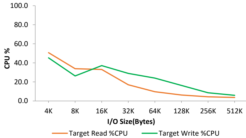
Figure 2 – iSCSI Target CPU Utilization vs. I/O size
